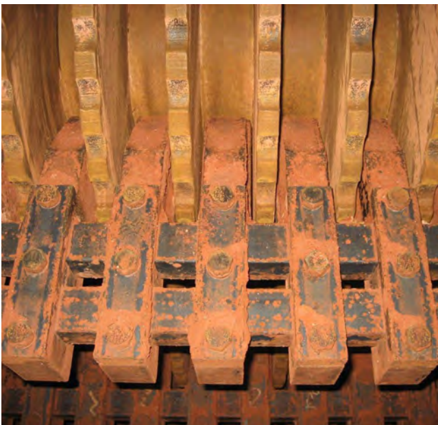
Integrated scraper system for difficult wet/sticky applications
